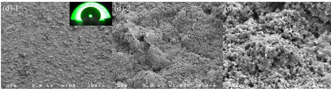
Figure 5-6: Different magnification SEM images showing the coating morphology before and after tape test. Sample P40 C60 (40/60 wt% PIP/CB blends, 12.5 mg mL -1 ) was sprayed on 6×6cm 2 butyl rubber substrate using 25 mL of suspensions. (a) UV cured and before tape test; (b) UV cured and after tape test; (c) not UV cured and before tape test and (d) not UV cured and after tape test. Optical image of the hexadecane contact angles are inserted in the top-right corner of the SEM images.
